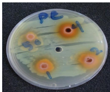
Figure, 5: Inhibition zones of Proteus spp. growth on Mueller-Hinton agar produced by ethanolic extract of Vitis vinifera , the peripheral four wells contained extract concentrations ( 50, 100, 200, 400 mg/ml) whereas the central well contained 0.1 ml of 96% ethanol
