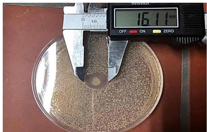
Figure 7. Agar diffusion test of SIS hydrogel shows 16.11 mm zoon of inhibition
